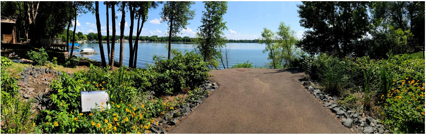
In Lindstrom, new or rebuilt city streets are made narrower when possible — a strategy that reduces stormwater runoff and cuts city maintenance costs. Linden Street was made narrower where it dead-ends at South Lindstrom Lake. It's flanked by a stormwater treatment system with rain gardens.
