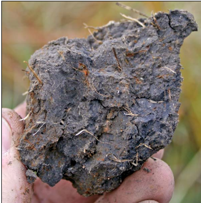
Figure 21. Redox features can be small and difficult to see within a dark soil layer.
