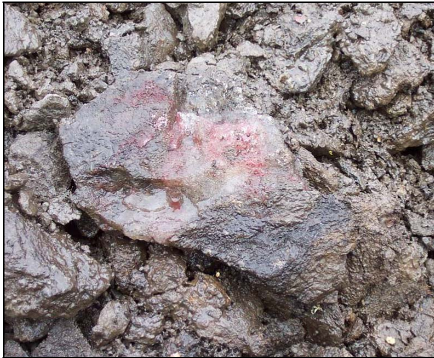
Figure 43. When alpha, alpha-dipyridyl is applied to a soil containing reduced iron, a positive reaction is indicated by a pink or red coloration to the treated area.
